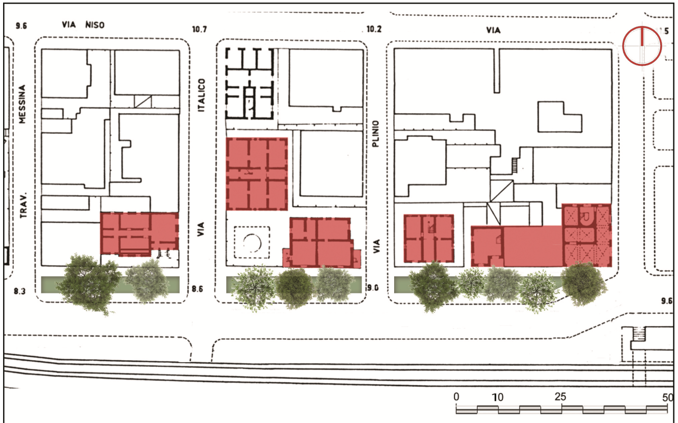
Fig. 6, Analysis and proposal for intervention n. 1/3; elements positioned parallel to the curtain of buildings (trees or photovoltaic panelling). Detailed plan.
