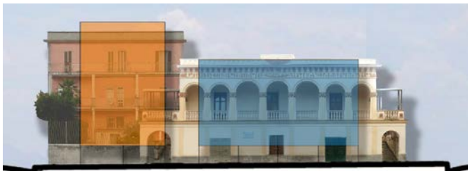
Fig. 12, Analysis and proposal for intervention n. 3; shielding by shielding by semi-transparent coloured solar glasses, study of the visual perception of the site
