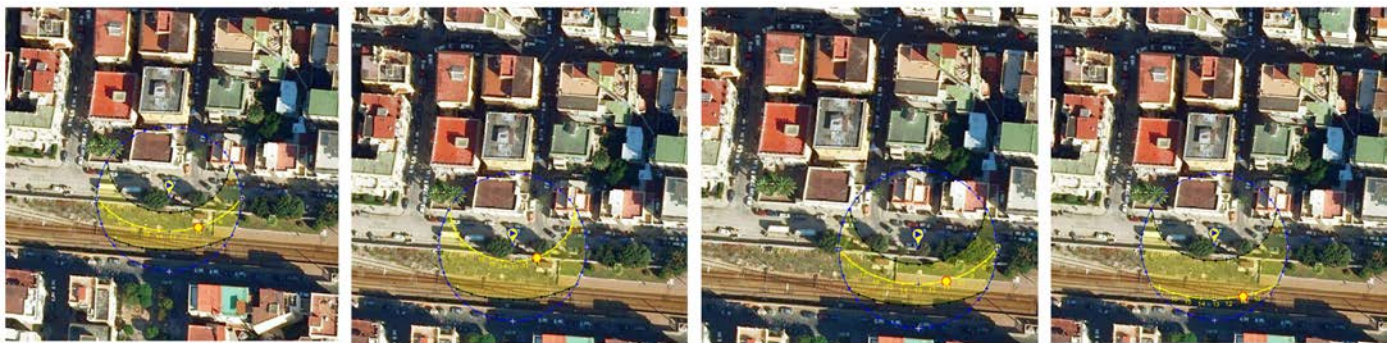
Fig. 2, Sun-path diagrams of Giusso district. The solar irradiation on the curtain of the buildings examined, particularly strong in the southern exposure
